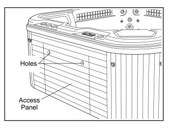
To replace the access panel, insert the bottom of the access panel into the lip of the spa base. Push the access cover in until it is securely in place.
